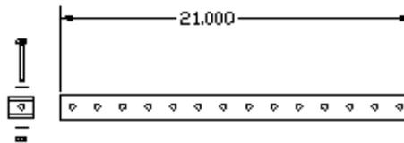
Step 3: Bolt 21" tube onto 36" tube through 2nd hole from one end. Use (1) 2" hex bolt and (1) flat washer. **NOTE: FOR A BETTER APPEARANCE, KEEP ALL BOLT HEADS ON SAME SIDE.**
