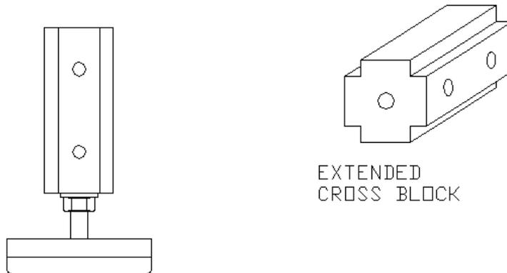
Step 4: Install foot assembly into (6) 13.5" long tubes. Use (1) 2-1/4" hex bolt, (2) flat washers (one per side), and (1) nylon insert lock nut per assembly
