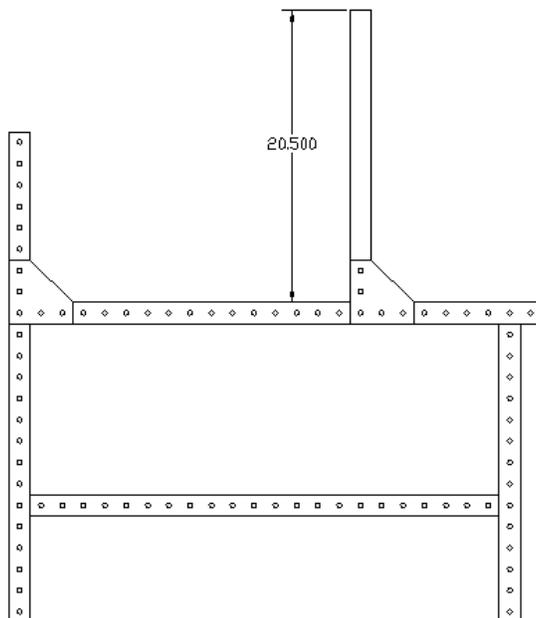
Step 8: Using (1) 5 hole gusset plate attach 15" perforated tube to 36" tube. 15" Tube should mount so that there are 4 open holes between the 5 hole gusset plates as in the picture below. Use (4) 2-1/4" hex bolts, (8) flat washers (one per side) and (4) nylon insert lock nuts. **NOTE: MAKE SURE TO ASSEMBLE (1) LEFT AND (1) RIGHT ASSEMBLY**
