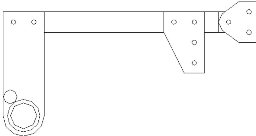
Step 5: Install pivot roller assembly onto 15" perforated tube located on side frame assembly. Use (2) 2-1/2" hex bolts, (4) flat washers, and (2) nylon insert lock nuts. Adjust the height of the rubber capped hex bolt so the 15-3/4" slotted beam is level to the ground.
