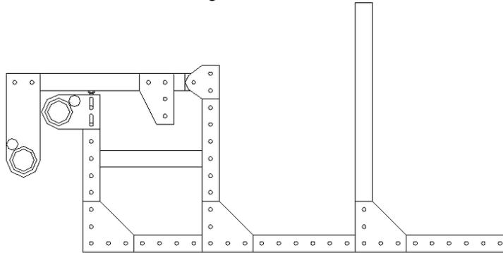
Step 6: Attach one ball stud to 4 hole gusset plate and secure with (1) nylon insert lock nut. Install the other ball stud with a flat washer into 5/16 T-nut located in 9" beam – see illustration for correct position. Make sure to use (1) flat washer between lower ball stud and 9" beam. Tighten lower mount.
