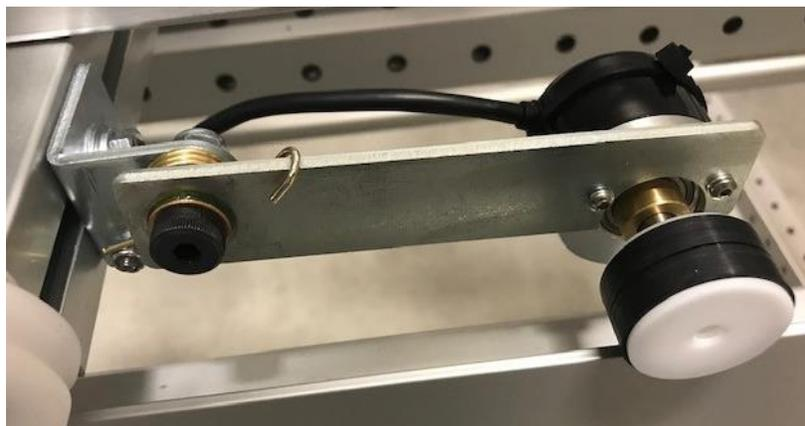
Step 2: Make sure the gold mounting plate of the channel lock is installed close to the left end of the t-slot rail (see picture below). If you are installing spring loaded encoders on an older machine, replace the (2) 1/4-20 x 1/2" Low Head bolts with (2) 1/4-20 x 1/2" Socket Head bolts.
