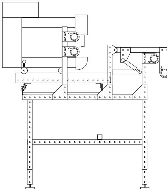
Step 20: Install large rubber bumpers onto 20.5" slotted beam on side of beam facing carriage assembly. Use (1) #10 x 3/4" socket head cap screw and (1) #10 t-nut. Adjust position of bumper so carriage contacts the bumper before hitting the end of frame. Install one bumper on each end.
