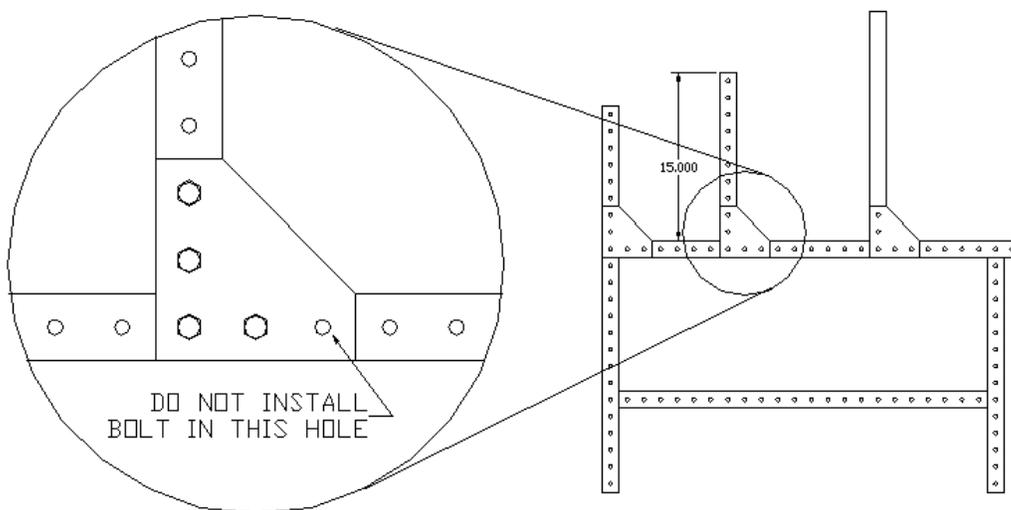
Step 9: Slide (1) 5/16 T-nut into any side slot of the 9" slotted beam. Install (1) 9" slotted beam between 15" tube and 34.5" tube through the 6th hole from open end of 15" tube. Use (2) 2" hex bolt and (2) flat washers. Position the 9" beam so that the slot with the T-nut faces the same direction as the 5 hole gussets.
