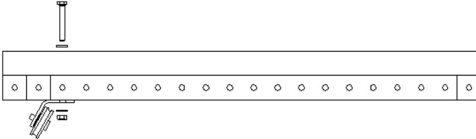
Step 4: Install lower carriage front wheel assembly onto 30" perforated rail tube thru the 4th hole from end of tube. Use (2) 2-1/4" hex bolts, (4) flat washers and (2) nylon insert lock nuts. **NOTE: SEE DRAWING FOR PROPER BRACKET AND WHEEL ORIENTATION.**
