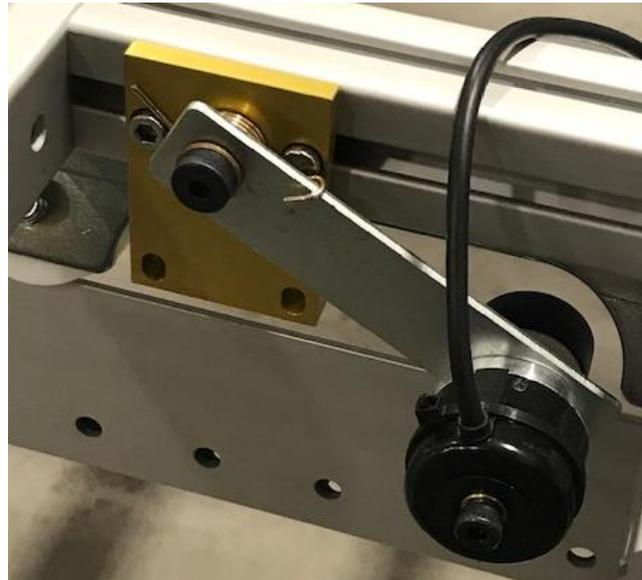
Step 4: Check to make sure the encoders move freely as the machine is moved left to right and front to back. The wheels of the encoders **MUST NOT** contact anything but the frame rail at any time and the encoder must pivot freely on the shoulder bolt. The wheel should lightly press against the rail with the help of the spring.
