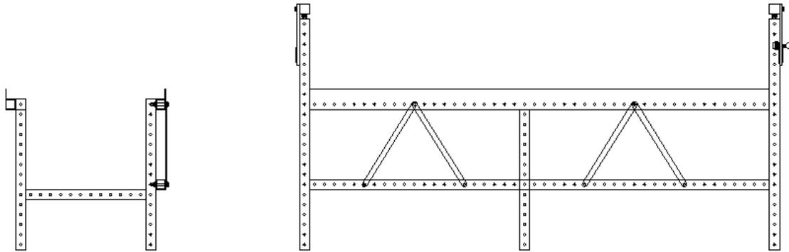
Step 9: Square lower carriage assembly to rail tubes. Insure that rails ride in the center of the wheels for smoothest performance. If rail to wheel relationship is consistent down the entire length of rail, adjust the lower carriage front wheel assembly. If the rail to wheel relationship differs as the carriage moves down the rail, adjust the long rail tubes by adding or removing washers to the round bar rail spacers.
