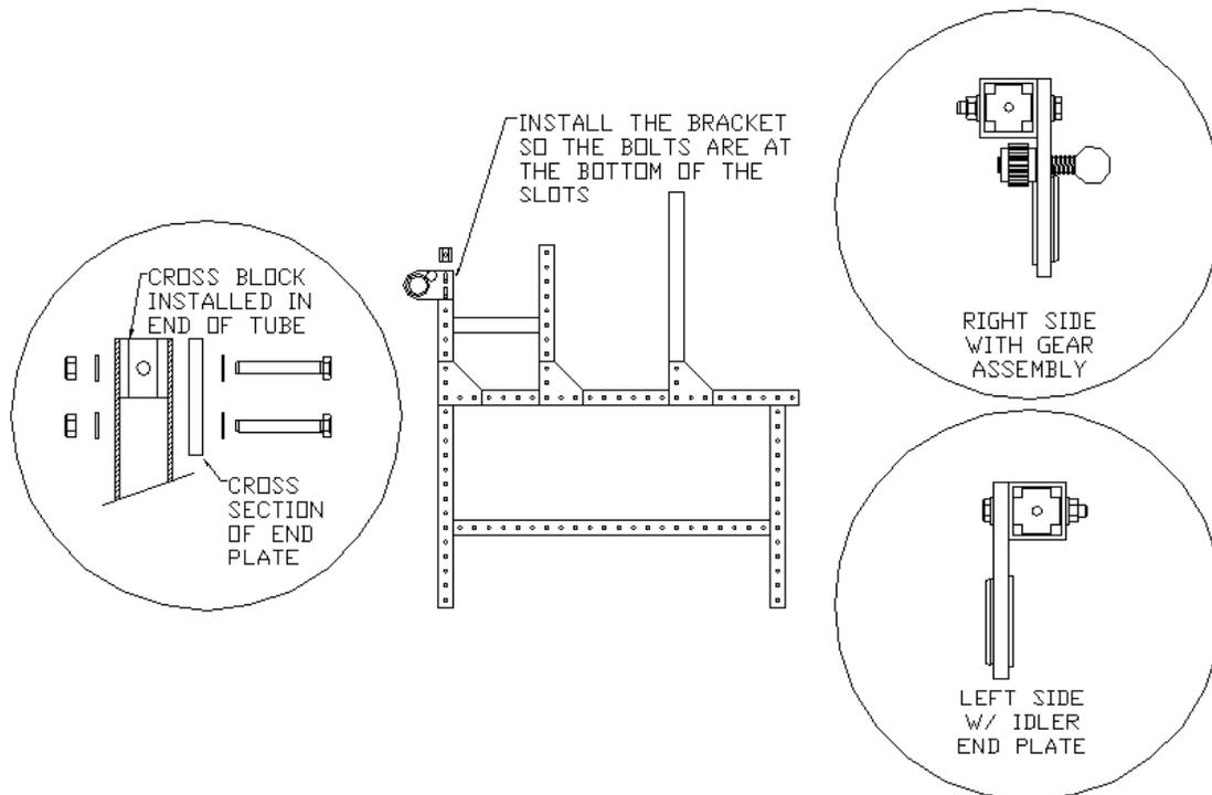
Step 11: Install (1) 1" hex bolt, (1) hex nut, and (1) flat washer into the end of the standard cross block. Install small rubber cap onto head of hex bolt. **NOTE: THE SMALL RUBBER CAP IS A VERY SNUG FIT AND SHOULD BE STARTED ON ONE OF THE POINTS OF THE HEX BOLT HEAD AND ROLLED ONTO THE ENTIRE BOLT HEAD. PRESS DOWN FIRMLY TO MAKE SURE RUBBER CAP HAS SEATED COMPLETELY ON THE BOLT HEAD.**
