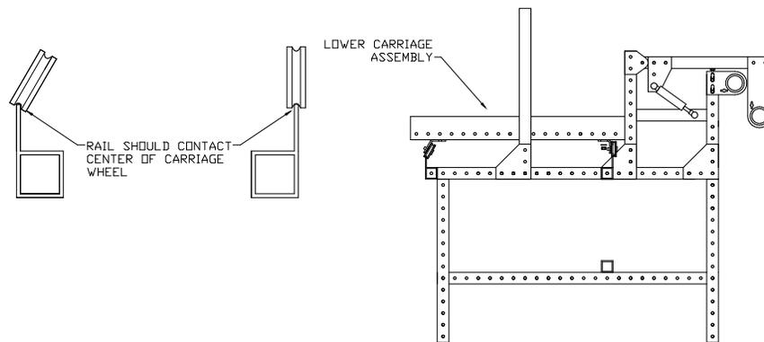
Step 10: Install (2) steel straps onto the long perforated rail tubes using (2) 2-1/4" hex bolts, (4) flat washers and (2) nylon insert lock nuts. See illustration for proper location and orientation.
