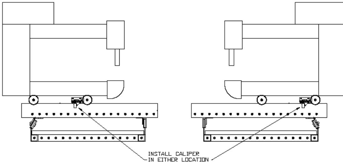
Step 2: Check to make sure the Y-axis caliper does not rub on the rail. A small amount of play in the caliper mount should be enough for adjustment. If it is rubbing, loosen the (2) 1/4-20 x 3/4 bolts from the previous step and hold up on the bracket while tightening the bolts.
