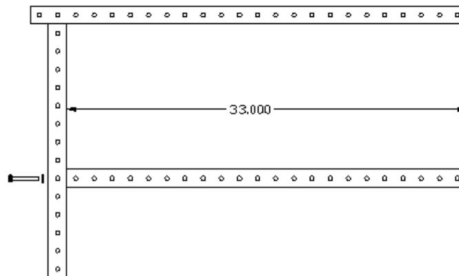
Step 5: Install 34.5" tube onto open end of 33" tube. Install into 6th hole from one end of 34.5" tube. Use (1) 2" hex bolt and (1) flat washer.
