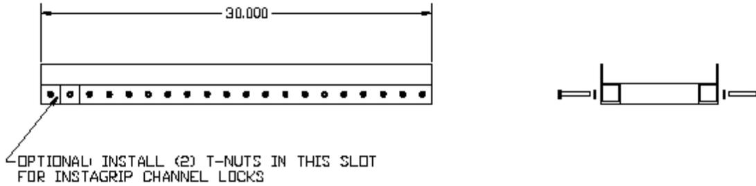
Step 2: Install a second 6" beam onto 30" perforated rail tube. Mount thru 1st hole on opposite end of tube. Use (2) 2" hex bolts and (2) flat washers
