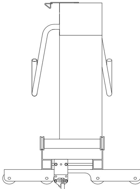
Step 6: Slide the X-axis caliper assembly as far to left side of the slot as possible, but do not allow any part of the assembly to come in contact with the wheel bracket. Tighten the (2) 1/4-20 socket bolts and check to make sure the caliper locks and unlocks without contacting any part of the wheel bracket. Adjust as necessary.
