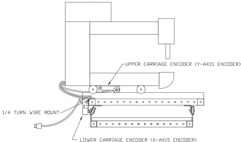
**Step 1: Install the upper carriage encoder (Y-axis) onto the rear aluminum wheel beam of the sewing head with the supplied bolt and nut. Make sure that the U on the spring end is hooked over the top of the encoder plate. Make sure the straight leg of the spring is resting on the small hex nut on the angle bracket. See the picture below. **NOTE: REMOVAL OF THE REAR WHEEL MAY BE NECESSARY TO INSTALL THE NUT.****
