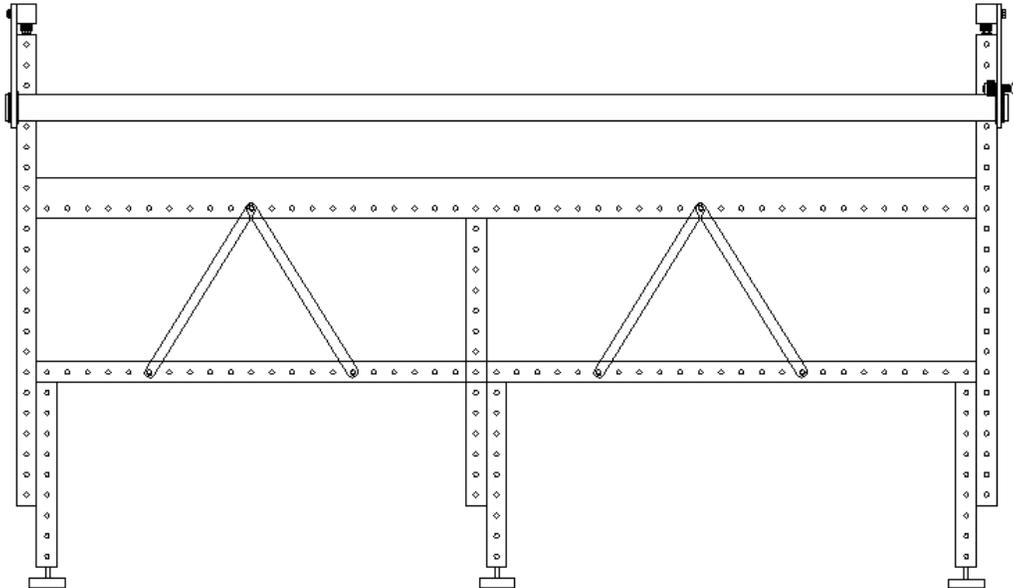
Step 18: Install table top between the long perforated rail tubes. Table should fit smoothly. Table should not be forced in between rails or damage may occur.
