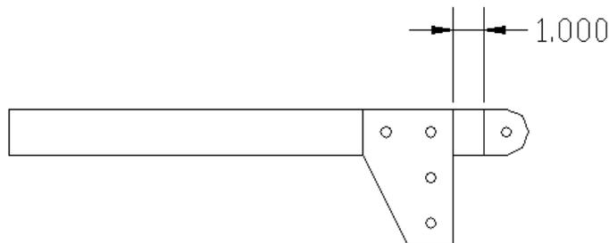
Step 3: Install top fabric roller end plates with and without gear assembly onto open end of 15-3/4" slotted beam - flush to end. Use (2) 1" hex bolts, (2) lock washers, (2) flat washers, and (1) double T-nut.
