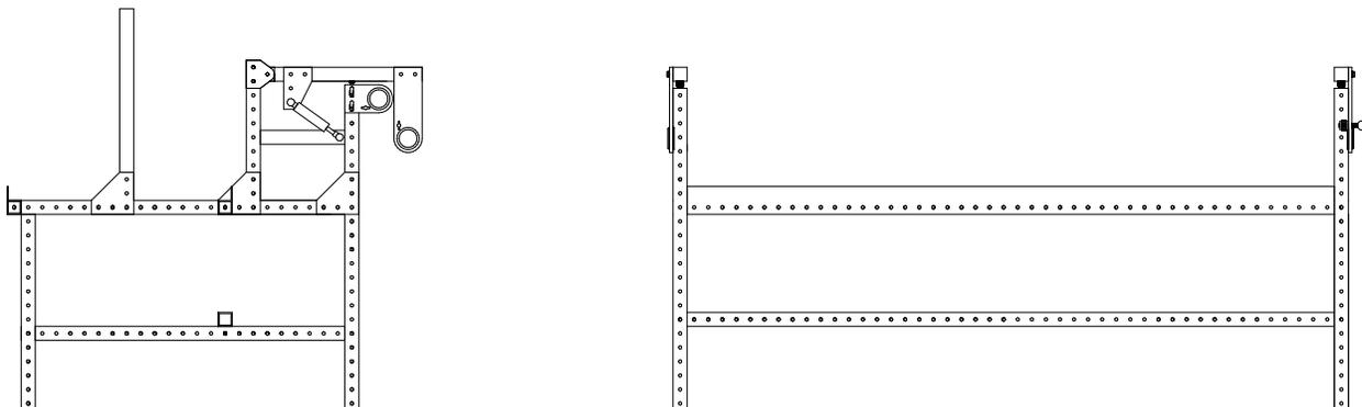
Step 4: Install (1) standard cross block (2 total) into each end of the 18" tube using (1) 2-1/4" hex bolt, (2) flat washer (one per side) and (1) nylon insert lock nut. **NOTE: INSTALL SO THAT HEX HEADS ARE FACING THE SAME DIRECTION ON EACH END.**
