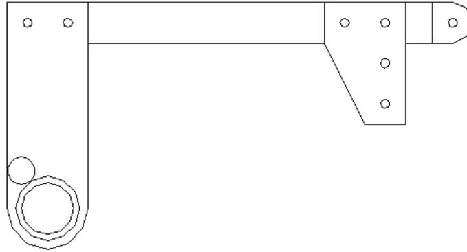
Step 4: Install (2) pivot arm brackets onto nub end. Use (2) pivot arm shoulder bolts and (2) plastic washers. Install plastic washer between pivot arm bracket and pivot nub.
