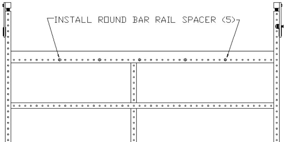
Step 8: Install (4) steel straps to lower tube and upper perforated rail tube using (6) 2-1/4" hex bolts, (12) flat washers, and (6) nylon insert lock nuts. See drawing for hole locations.
