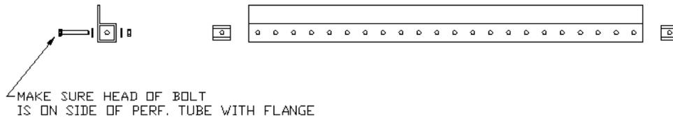
Step 2: Bolt long perforated rail tubes to side rail support frame assemblies using (2) 2-1/4" hex bolts and (2) flat washers to bolt the front rail through the 5 hole gusset plate and use (2) 2" hex bolts, and (2) flat washers for the other rail. **NOTE: SEE DRAWING FOR PERFORATED RAIL TUBE ORIENTATION AND LOCATION.**
