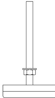
Step 3: Install machine feet into (6) extended cross blocks. Note only one end of extended cross block is threaded.
