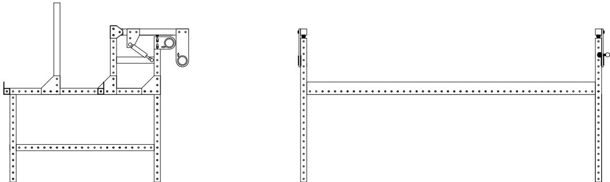
Step 3: Bolt long perforated square tube to side rail support frame assemblies using (2) 3-1/2" hex bolts, (4) flat washers, and (2) nylon insert lock nuts. **NOTE: POSITION TUBE DIRECTLY BELOW FRONT LONG PERFORATED RAIL TUBE.**
