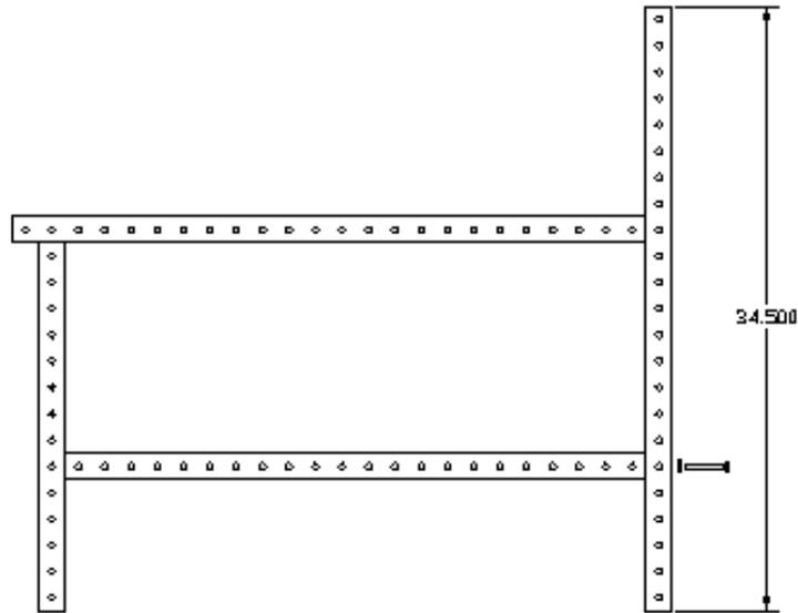
Step 6: Using (1) 5 hole gusset plate attach 36" tube to 34.5" tube. Use (5) 2-1/4" hex bolts, (10) flat washers (one per side) and (5) nylon insert lock nuts. **NOTE: MAKE SURE TO ASSEMBLE (1) LEFT AND (1) RIGHT ASSEMBLY.**
