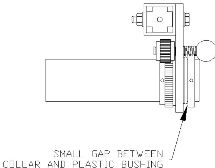
Step 15: Install the remaining roller tube into the bed roller end plates and install the (2) collars, one on either side of the plate, as shown below. Tighten the (3) set screws on each of the collars. Check to make sure the roller turns freely.
