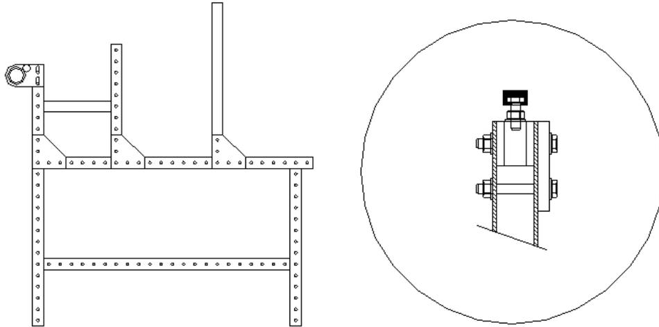
Step 12: Completed pro-frame left and right side rail support assemblies.
