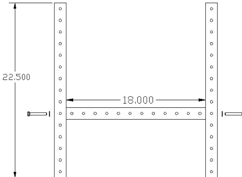
Step 6: Install the center leg assembly at approximately the center of the perforated rail. Use (1) 3-1/2" hex bolts, (2) flat washers, and (1) nylon insert lock nut to attach the assembly to the lower beam. Use (1) 3-1/2" hex bolts, (2) flat washers and (1) nylon insert lock nut to attach the leg assembly to each of the long perforated rails.
