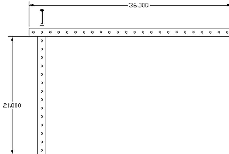
Step 4: Bolt 33" tube, from step 1, to 21" tube (9) holes down from connection to 36" tube. Use (1) 2" hex bolt and (1) flat washer.
