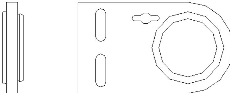
Top fabric roller end plate with gear assembly (Qty. 1)
