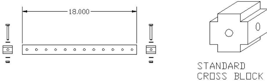
Step 5: Install 18" tube into 6<sup>th</sup> hole from the bottom of the (2) 22.5" tubes. Use (2) 2" hex bolts and (2) flat washers. The center leg assembly is now complete.
