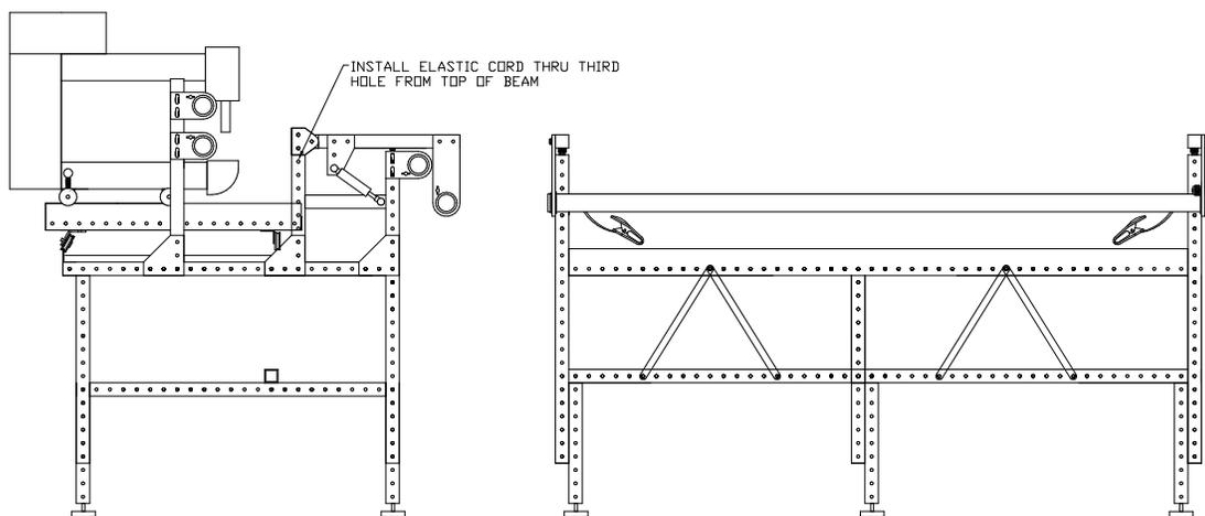
Step 22: Install the remaining (12) tubing end caps into any open square ends of the frame.
