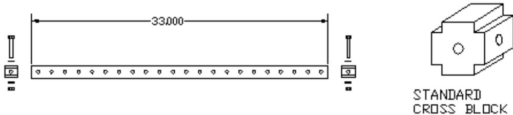
Step 2: Install a standard cross block into one end of the 21" tube using (1) 2-1/4 hex bolt, (2) flat washer (one per side) and (1) nylon insert lock nut.
